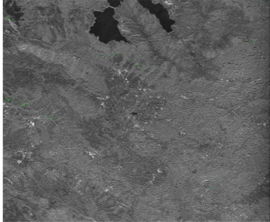
Fig. 2. Calibrated COSMO-SkyMed SAR image obtained by applying the GICAL processing scheme. A layover mask (in green) is also superimposed.
