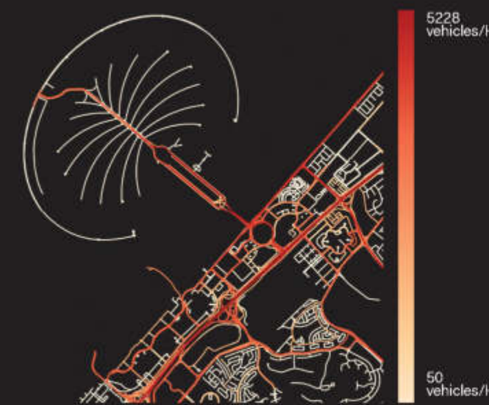
● TRAFFIC VOLUME The vehicular traffic flow, measured as for direction nearest to the subject sidewalk, can have a strong negative impact on the PLOS, especially if the traffic volume is substantial.
